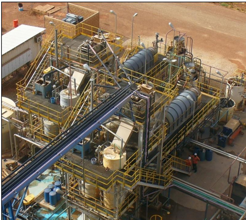
Figure 44: Acid Wash/Elution Circuit with Carbon Regeneration Kilns at Rear
